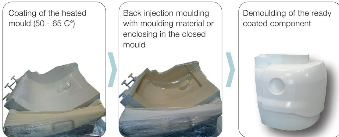
Advantage: A significantly faster production process without additional coating of the parts.
