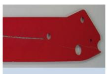
Production component after a 504-hour salt spray test.
