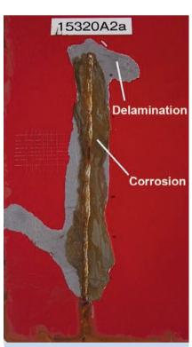
Evaluation of the corrosion and delamination from the scribe line after corrosion protection tests.
