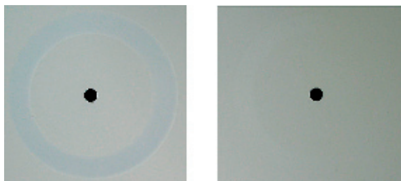
Figure 2: Significant difference after 300 load cycles – the standard powder coating (left) and the highly abrasion-resistant powder coating (right)
