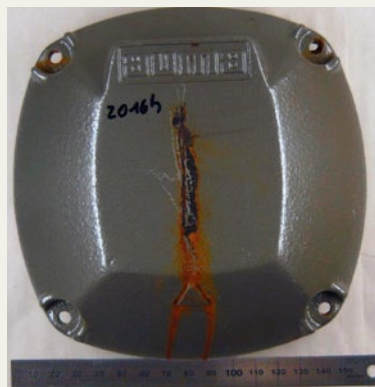
Salt spray test on cast iron (zinc-phosphated) after 2016 hours.
