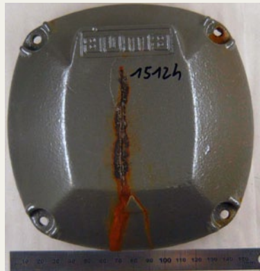
Salt spray test on cast iron (zinc-phosphated) after 1512 hours.
