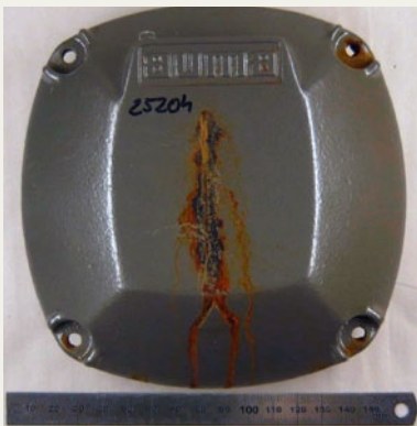
Salt spray test on cast iron (zinc-phosphated) after 2520 hours.
