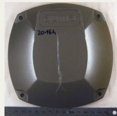
Salt spray test on die cast steel (zinc-phosphated) after 2016 hours.
