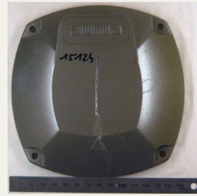
Salt spray test on die cast steel (zinc-phosphated) after 1512 hours.
