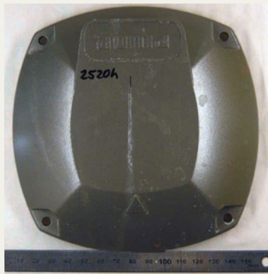
Salt spray test on die cast steel (zinc-phosphated) after 2520 hours.
