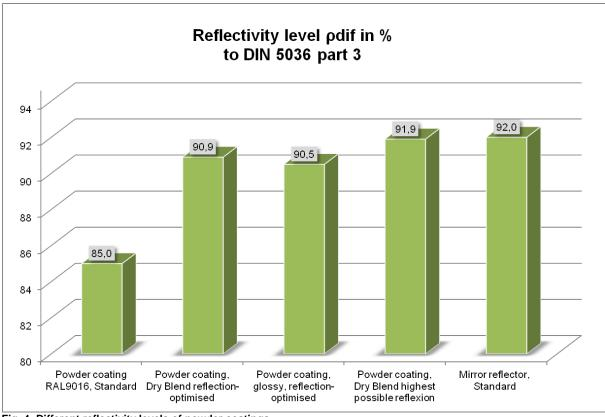
Fig. 4: Different reflectivity levels of powder coatings
