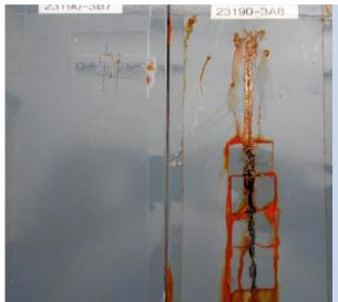
Corrosion protection results for the two-layer coating of UR1407 and UR1984 with a total coating thickness of approximately 140 µm after a 720 hour condensation test (left) and 1000 hour salt spray test (right); Substrate: blasted steel (right), Sa 2.5,  $Rz = 30 \mu m$ , creepage: <2 mm, subsurface corrosion: approximately 1 mm, no bubbles on the surface or cut edge
