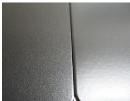
Figure 2: The sparkling effect of new dry blend powder coatings (right) is significantly reduced in comparison with standard systems (left).
